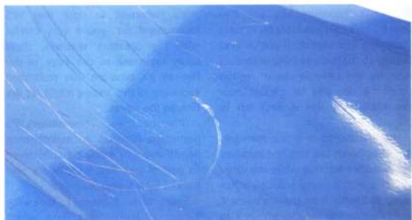
The right-hand side of this test panel is protected with film; here you can see how resistant it is to scratching.
