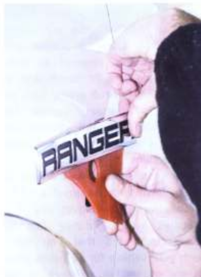
Left Minor trim items are temporarily removed. Right The film is cut using templates.
