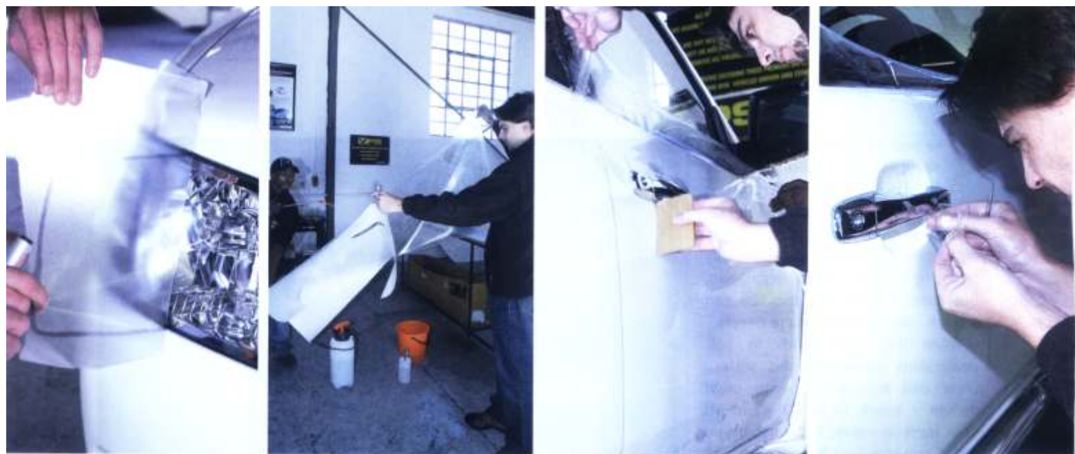
These pictures show the entire fitment sequence, from creating a template all the way through to the intricate final trimming.
