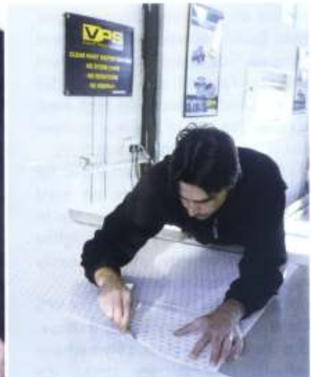
Left Minor trim items are temporarily removed. Right The film is cut using templates.
